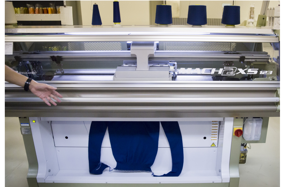
Fig: Whole garment knitting with Shima Seiki's machine. https://about.newenergyfinance.com/blog/these-hi-tech-knitting-machines-will-soon-be-making-car-parts/
