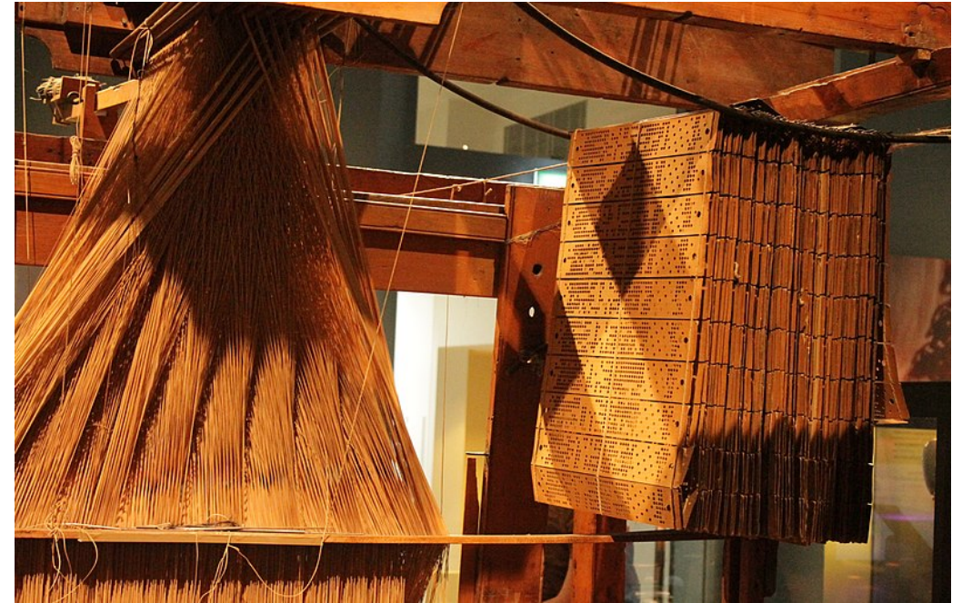
Fig: Punchingcards on a Jacquard loom, copyright wikimedia
